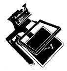
The jacket hold-down is a very important piece of equipment, as it must hold the nylon fabric securely. Because most jackets printed are multiple layer garments (lined), just putting adhesive on the platen will not hold the top layer of the garment in place.
